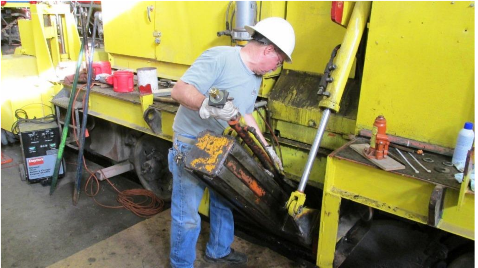
With the lift-cylinder now attached to the pivot arm, Mike H. installs the extender cylinder
