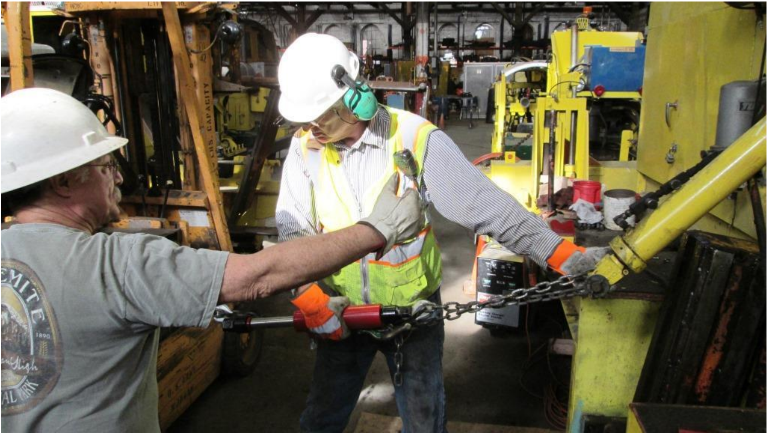
Mike H. and Steve hook up a chain and a come-along to the lift cylinder of the regulator
