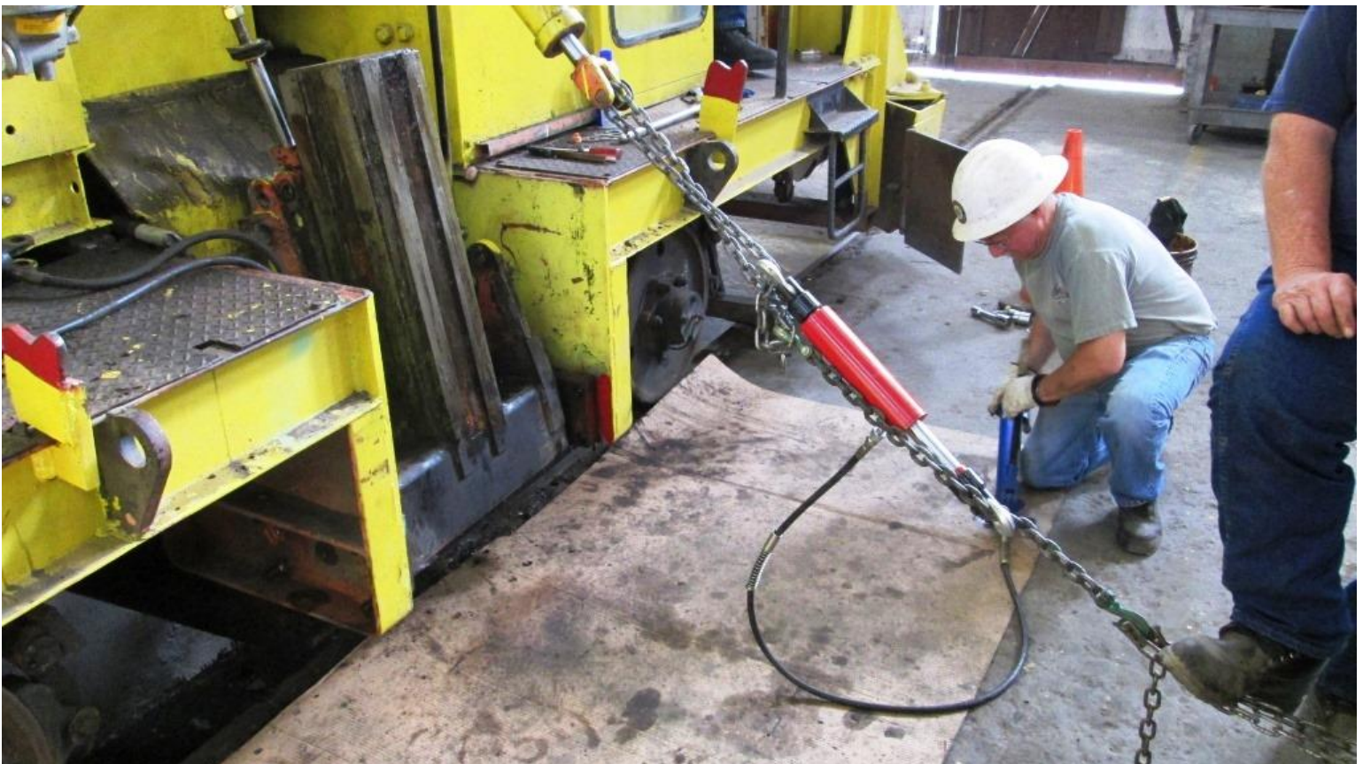
Mike H. uses the hydraulic come-along to pull the lift cylinder rod out
