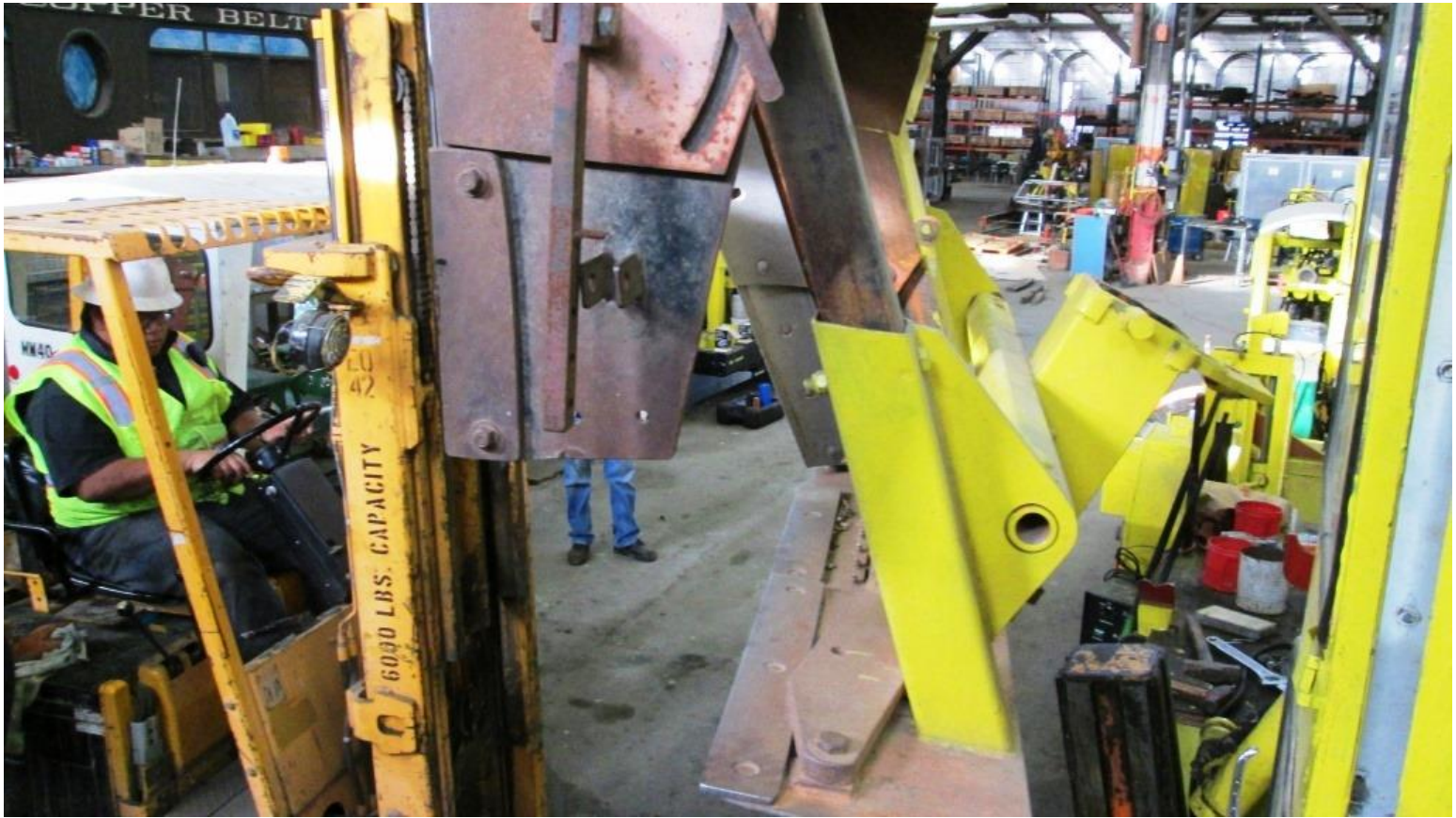
...And maneuvers to line it up with the pivot arm
